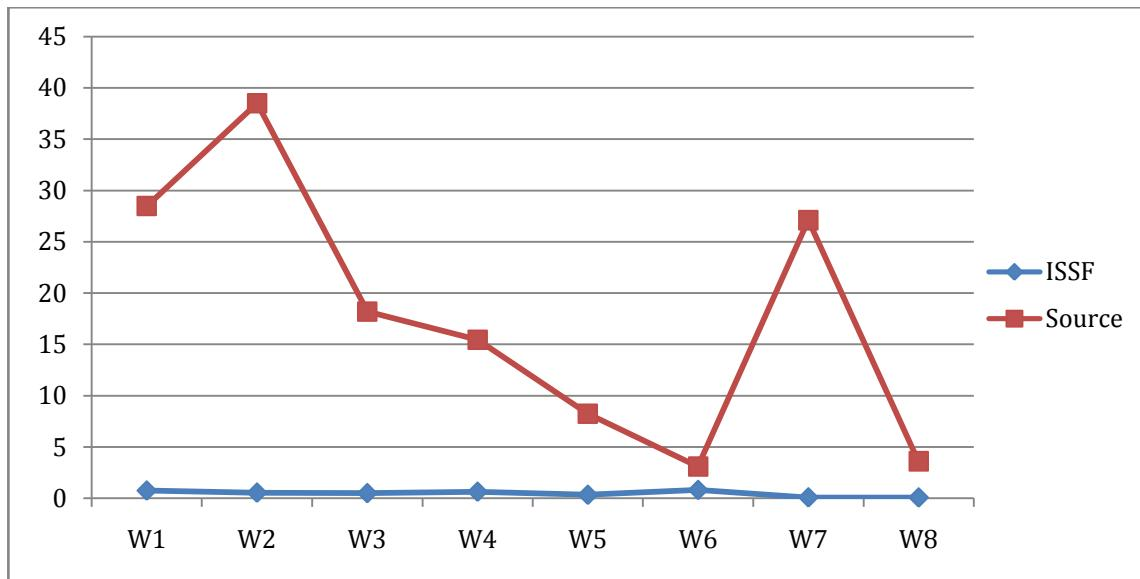
Refer to table # 5 for details. It is to mention that the turbidity of source water was changeable due to the weather condition, if there was raining the turbidity was to be increased due to small flooding.
