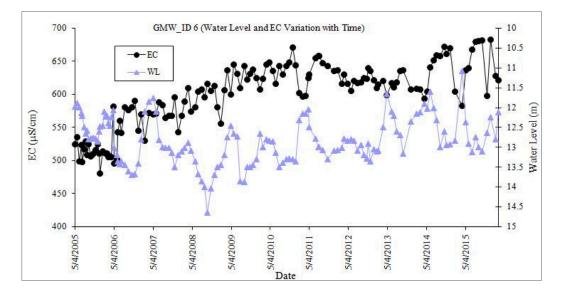
Figure 10. GWM\_ID 6 Time Series Water Table Fluctuation
