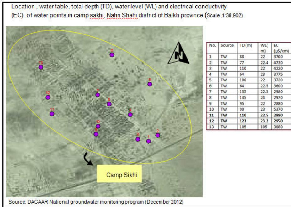
**Figure 3 Groundwater level and salinity distribution**
