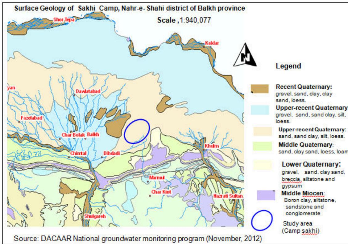
Figure 2 Surface Geological setting of the survey area (Balkh Province)
