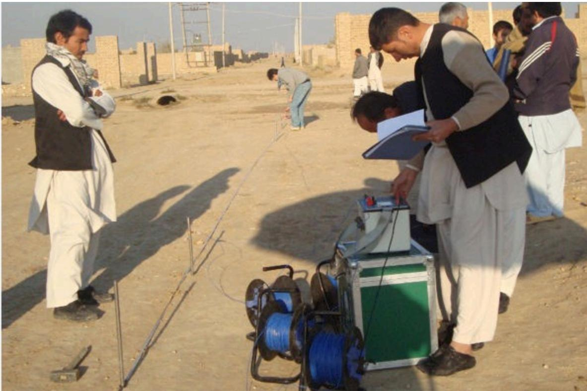
Figure 1 Recording VES profile field data using SYSCAL Pro resistivity meter
