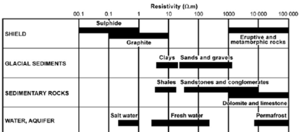
Figure 5 Resistivity scale for water and rocks
