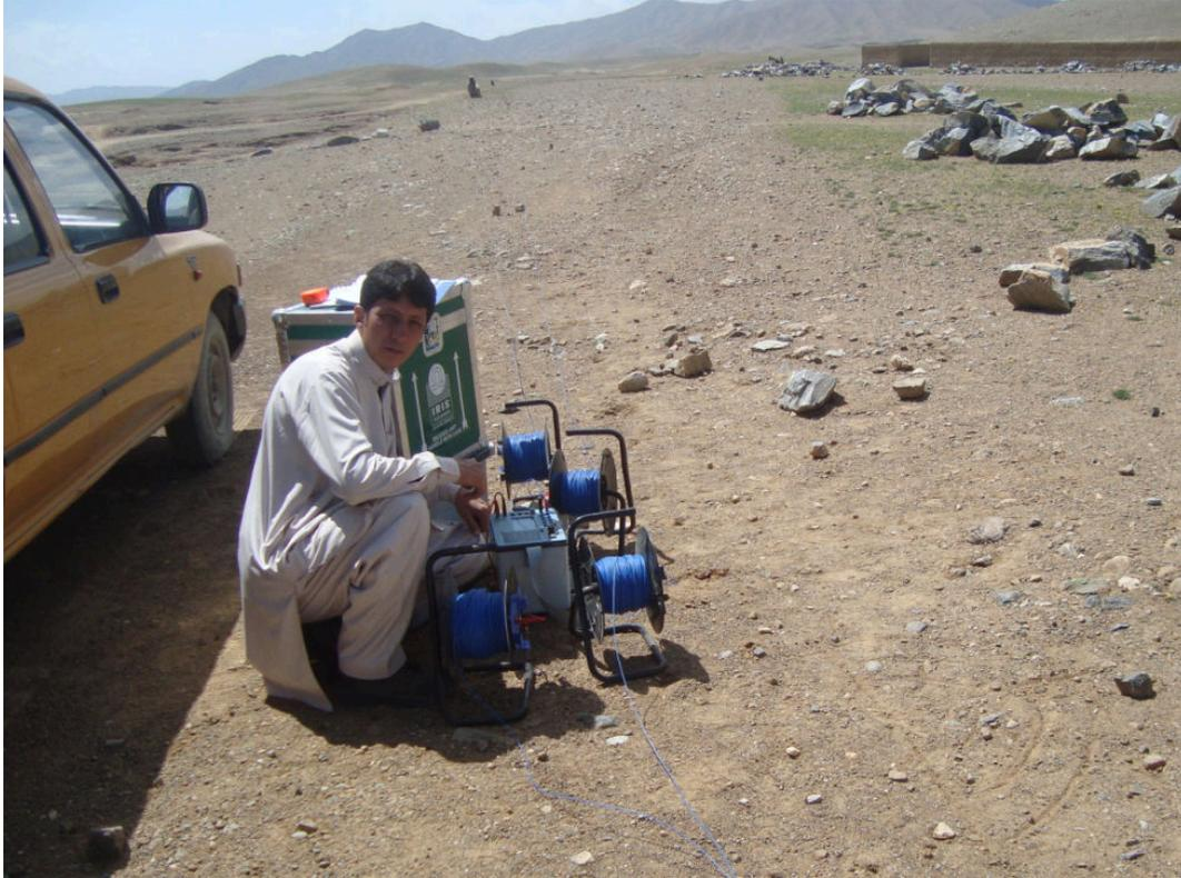
Figure 2, Recording VES profile field data using SYSCAL Pro resistivity meter
