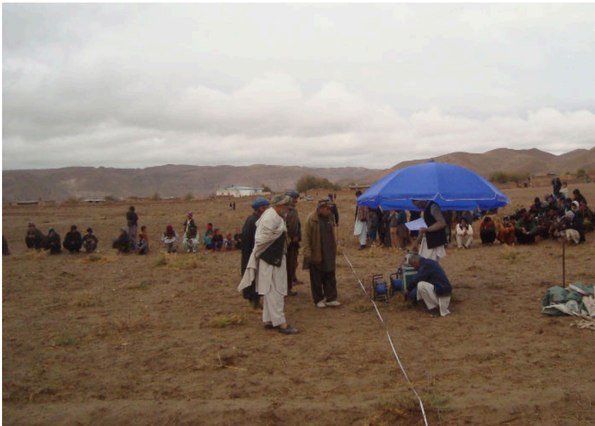
Figure 1 Recording VES profile field data using SYSCAL Pro resistivity meter
