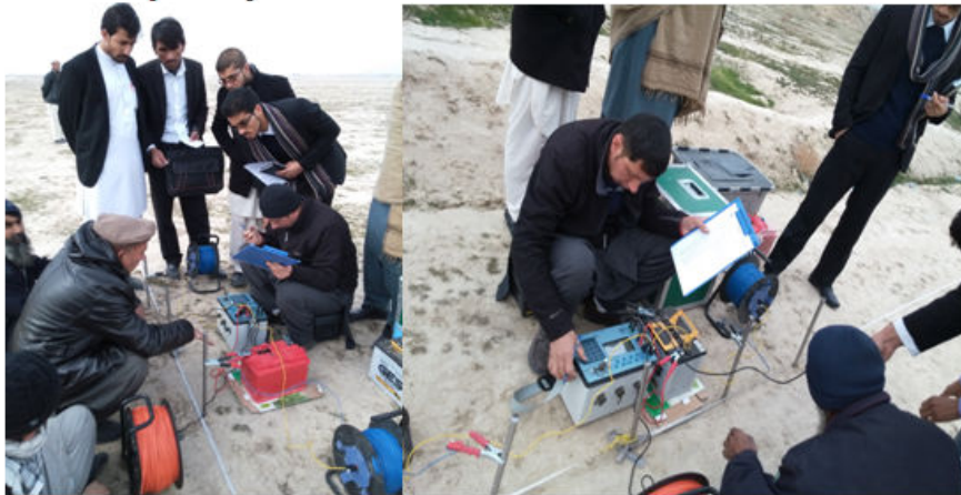
Figure 3 Measured Field Data By SYSCAL Pro Resistivity Meter
