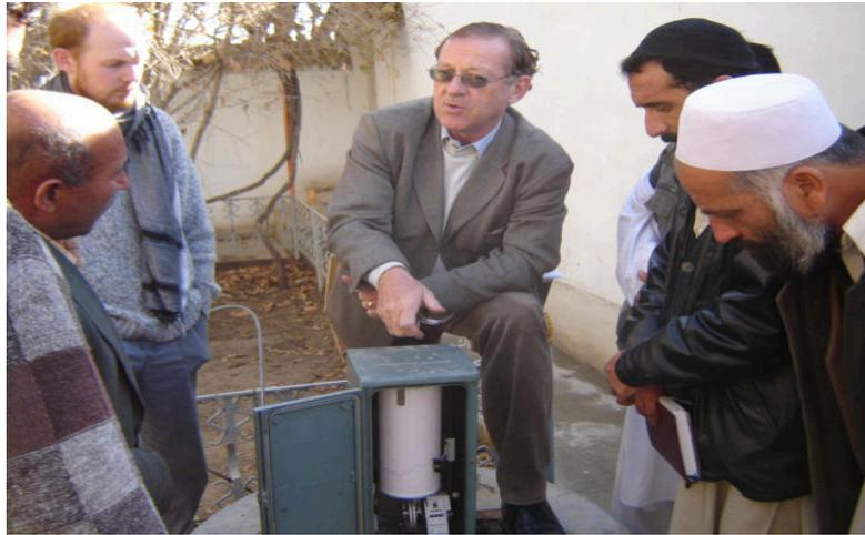
Fig. 9 SEBA Water Level Recorder.
