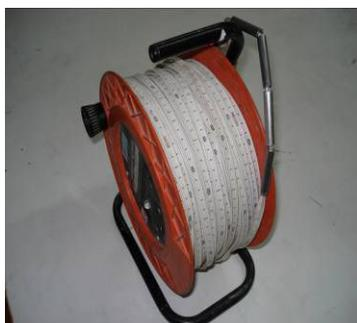
Fig.4. Water level Indicator.
